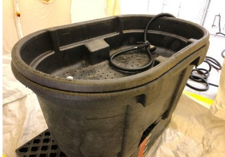
Canine Unit with Hose and Drain System
