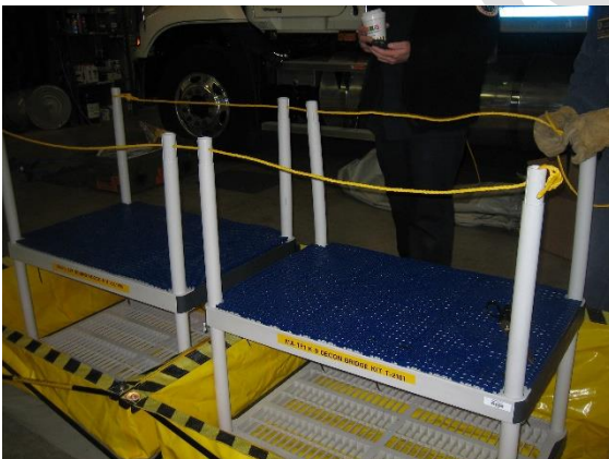
MA TF1 Elevation of shelves, non-slip flooring, rope visual barriers, TVI pools
